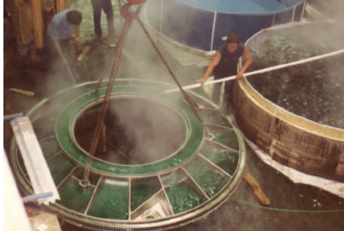
Photo: 1 Beer Filling Machine being plated with MB
