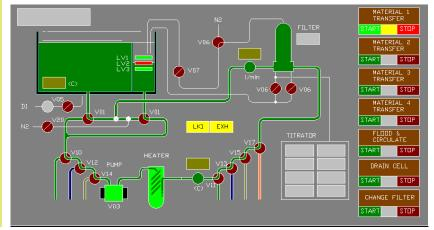
Detailed Display screens like this one provide the operator with a complete picture of the tool operations. Using standard Windows menus, the operator can quickly navigate between the different programs to control all aspects of the wafer processing.
