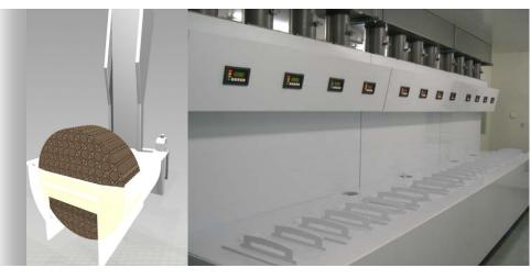
Stapleton Technologies provides several aqueous metalization tools for wafer processing. These range in size and complexity depending on the needs of the Fab. Production and tool quality requirements determine the complexity and material cost which directly effect the cost to deliver these systems.
