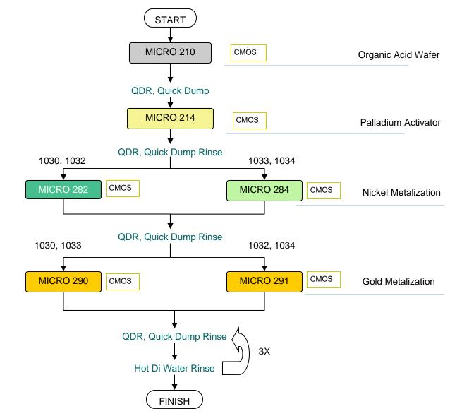
The process sequences described on these two pages summarizes the different methods of metalizing Aluminum and Copper with nickel and gold for solder and wirebond interconnect.
